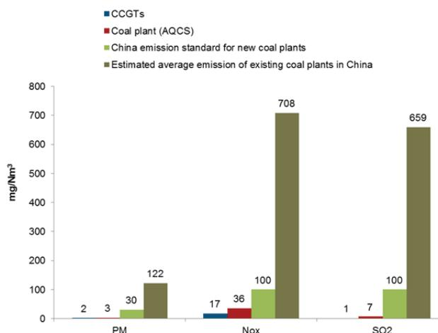
Source: Emission rates from gas-fired CCGT and coal-fired units with advanced AQCS are provided by Burns & McDonnell based on the most advanced available technologies. China's emission rate standards for new coal plant (effective 1 January 2012) are from China's Ministry of Environmental Protection. The average emission rates from China's existing coal plants are based on TLG analysis.
